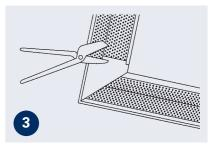
Insert further lengths, allowing a 25mm overlap. At corners, cut to 45° with tin snips and butt together.
