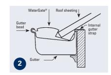
Position WaterGate® as shown so the flat edge slips up under the roof's edge and is supported beneath by the internal gutter straps.
