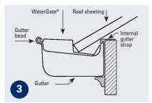
This will allow you to insert the outer 'v' shaped edge into the gutter's outer edge bead, clipping the WaterGate securely in place.
