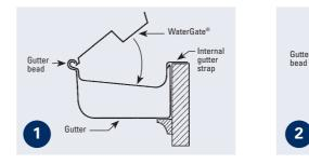
Insert the small 'v' shaped end of WaterGate® into the gutter's outer edge bead.
