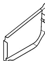
Gutter Stop Ends Zinalume® or Colorbond® Finish
