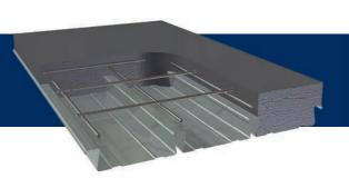
Fielders RF55® is a traditional flat pan or 're-entrant' profile that provides unmatched performance in suspended concrete slabs. RF55® is used in both concrete and steel frame construction and utilises patented technology to achieve superior spanning capabilities, less deflection and greater composite strength than similar re-entrant profiles. RF55® comes complete with a range of accessories allowing for easy suspension of ceilings and services.
