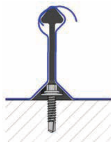
Figure 1.8: FreeForm™ detail of lap before seaming.
